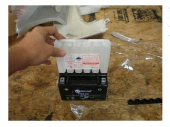
Pull all materials out of the box. Pull the red sticker off of the top of the battery.
