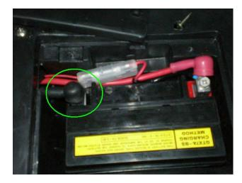
Charge the battery at no more than 7amps. If you use a charger that is set to a higher amperage, you will overcharge the battery and possibly cause it to explode.
