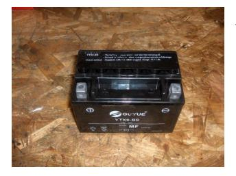
If the acid does not go into the battery, pierce the top of each vial with a thumb tac.
